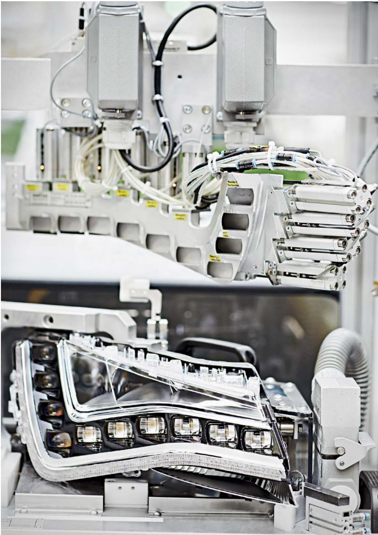
Increasingly complex: assembly of a full LED headlamp in Lippstadt/Germany.
